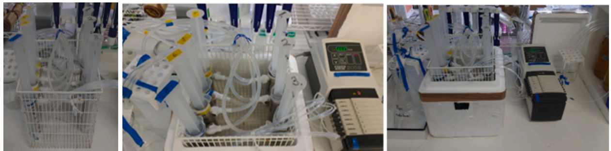
Fig. 4. (a) Schematic and (b) Photographs of the syringe sand columns with single-pass flow system for loading biofilm ( Bacillus mojavensis grown in Nutrient Broth E).
