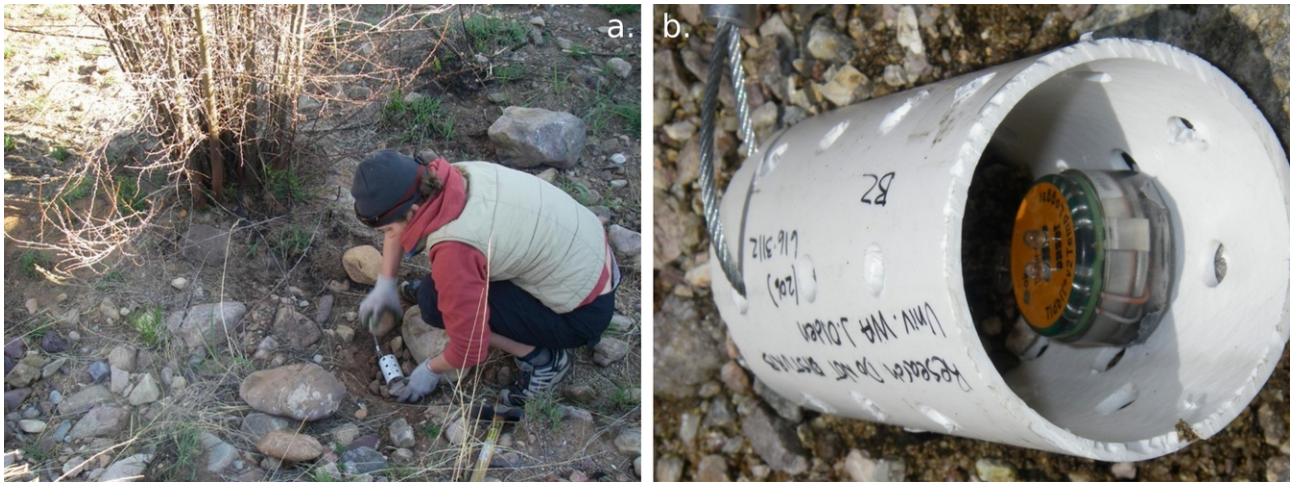
Figure 3.2: Conductivity sensor being put in place in 2010 (a) and close-up of the sensor in its protective white casing (b). Photos courtesy of Meryl Mims.
