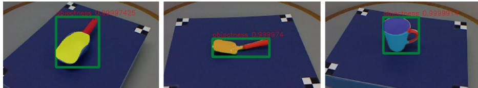
(a) Segmented image from (Chu et al. , 2019). Red parts afford to grasp, yellow parts afford to scoop, orange parts afford to support, deep blue parts afford to contain, and blue parts afford wrap-grasping.
