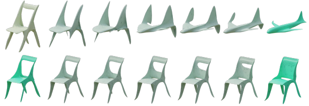
Figure 8. 3D meshes in each row are sliced from the same 4D tetrahedral mesh, they have different shapes and topologies.
