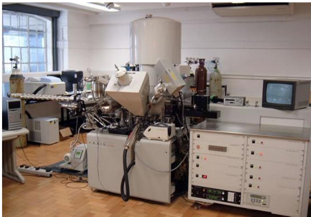
Figure 2.11: Kratos Axis Ultra DLD X-ray photoelectron spectrometer used in the current study.
