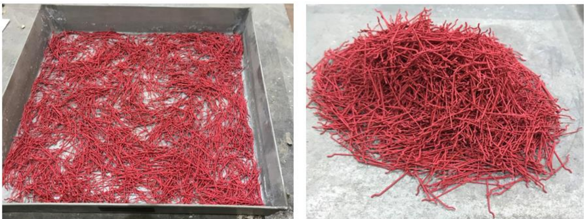
Figure D-4:Color-coded steel fibre; (the 30 mm long, 0.55 mm diameter)
