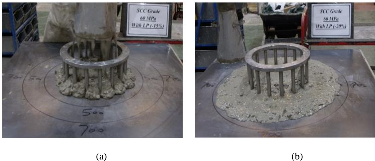
Figure 6.24: Flow and passing ability of SCC mix (a)C60 (iii) (b)C60 (iv)
