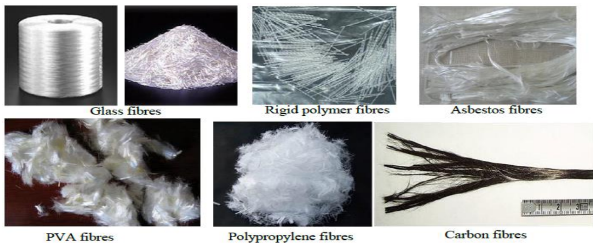
Figure 2.10: Different type of fibres used in concrete reinforcement
