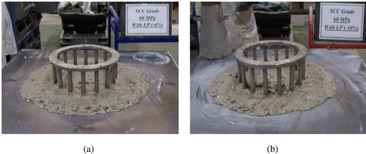
Figure 6.23: Flow and passing ability of SCC mix (a)C60 (i) (b)C60 (ii)
