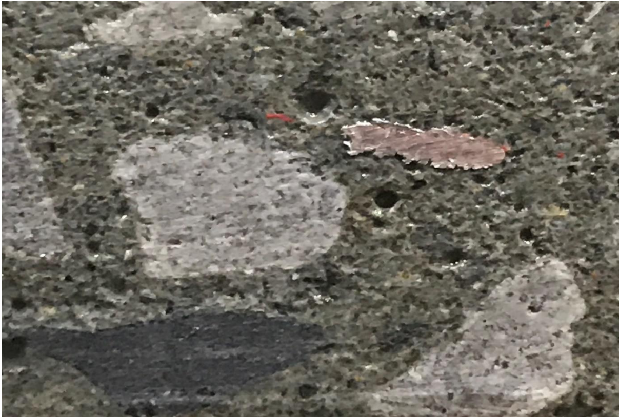
Figure D-3:Section of Cut the hardened of SCSFRC in the flow test
