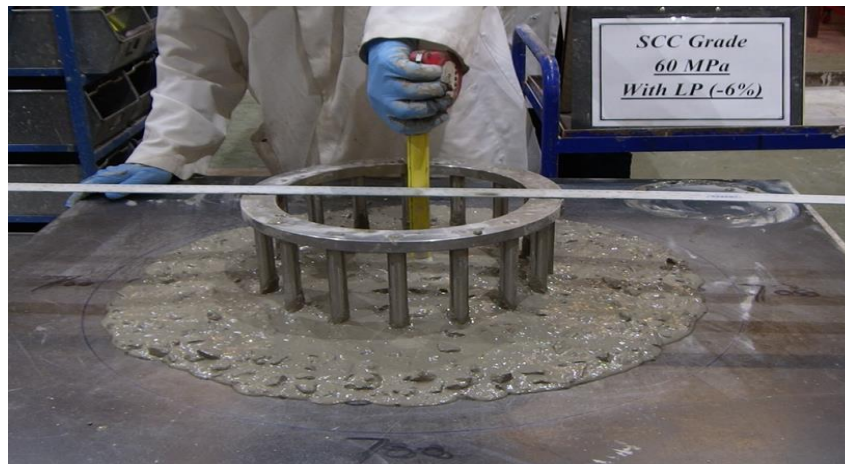
Figure 6.14: J-ring test (blocking step) SCC mix
