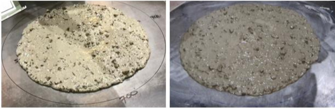
Figure 7.4: Horizontal spread of SCC and SCSFRC mix: C30 (Mix 1) (Left), C50 (5) (Right)
