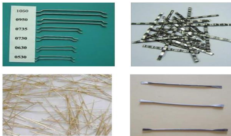
Figure 2.9: Different types of steel fibres used in reinforced concrete
