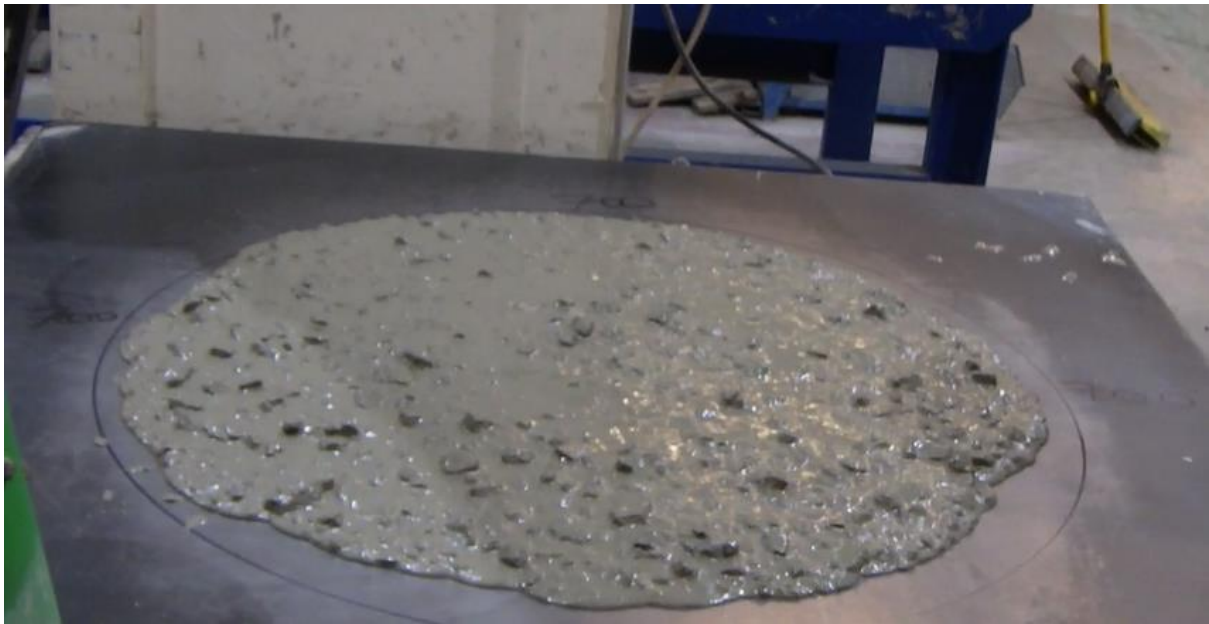
Figure C-5: Flowing ability of SCC mix: C70
