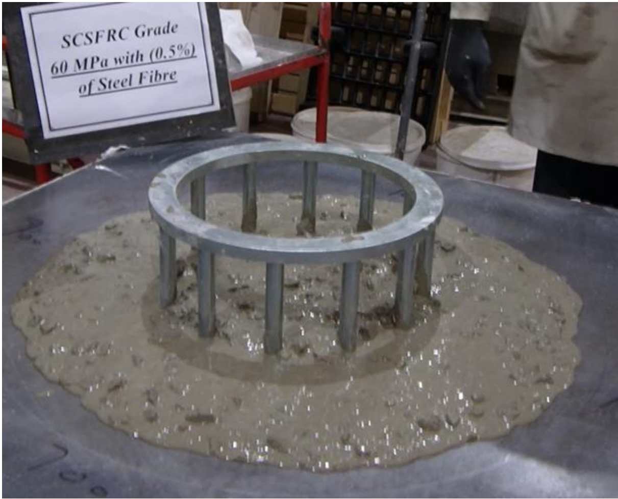
Figure C-12:Flowing and passing ability of SCSFRC mix: C60
