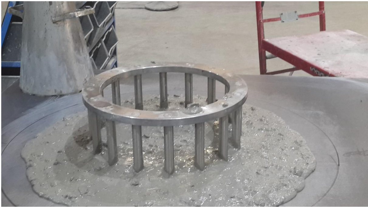
Figure C-2:Flowing and passing ability of SCC mix: C40
