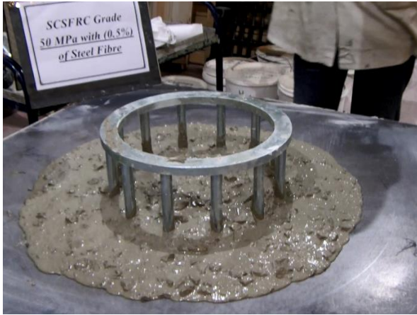
Figure C-11: Flowing and passing ability of SCSFRC mix: C50
