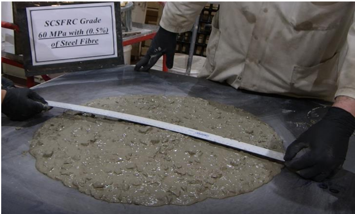
Figure C-11: Flowing and passing ability of SCSFRC mix: C50
