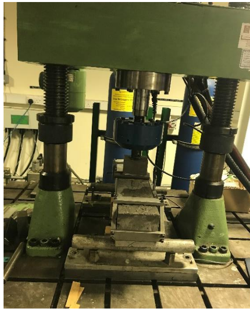
Figure 7.24: Beam specimen used for TPB test
