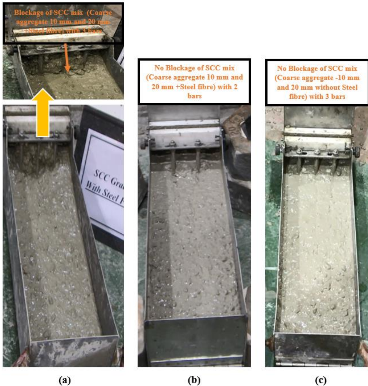
Figure 7.20: Flow, pass and fill-ability of SCSFRC mix: C40 (a) with 3 bars, C40 (b) with 2 bars, C60 (c) with 3 bars (size of coarse aggregate with 50 % of 10mm and with 50 % of 20mm)
