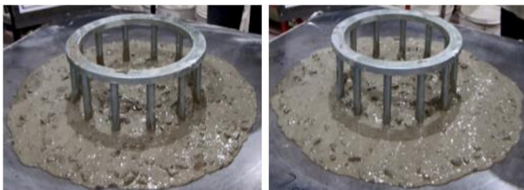
Figure 7.5: Flow and pass-ability of SCSFRC mix: C50 (Mix 5) (Left), C70 (Mix 8) (Right)
