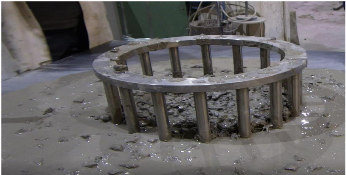
Figure C-10:Flowing and passing ability of SCSFRC mix: C40 *
