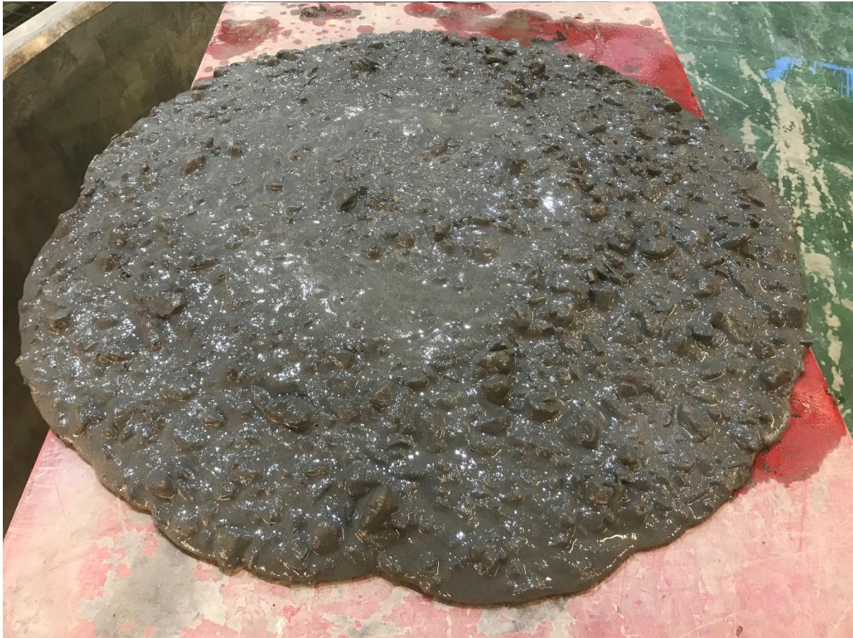
Figure D-1:Hardened of SCSFRC in the flow test
