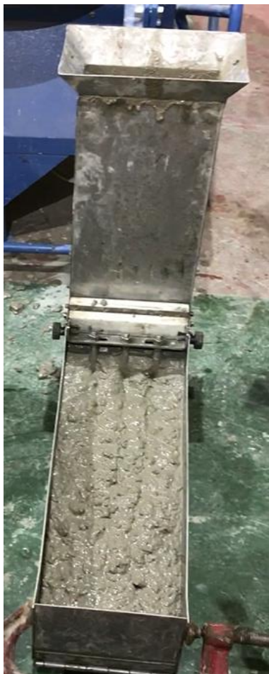
Figure C-4:Flowing and passing ability of SCC mix: C60
