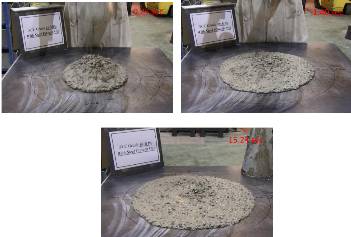
Figure 8.7: Experiment of slump flow test for SCSFRC (0.5% vol fibre)
