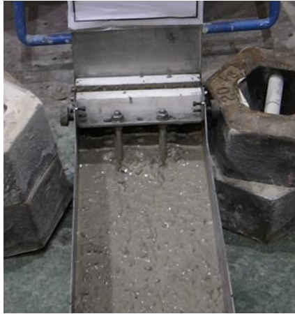
Figure C-7: Flowing , passing and filling ability of SCSFRC mix: C40
