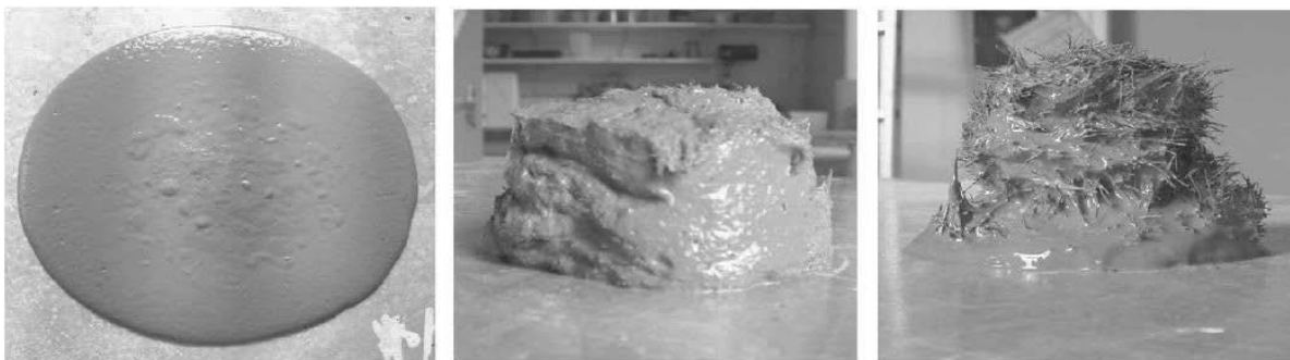
Figure 2.11: Effect of increasing the fibre factor ( v_f \cdot l_f / d_f ) on the consistency of a cement paste mixed with fibres (Martinie, Rossi and Roussel, 2010)
