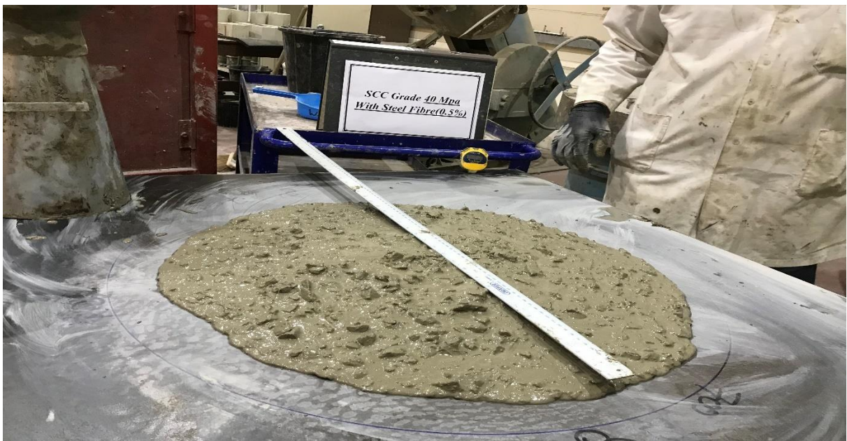
Figure C-7: Flowing , passing and filling ability of SCSFRC mix: C40
