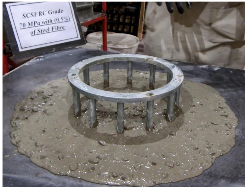
Figure C-13:Flowing and passing ability of SCSFRC mix: C70
