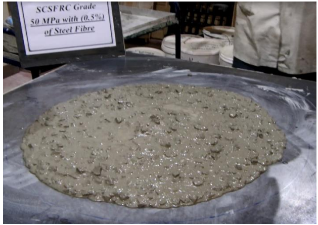
Figure C-11: Flowing and passing ability of SCSFRC mix: C50
