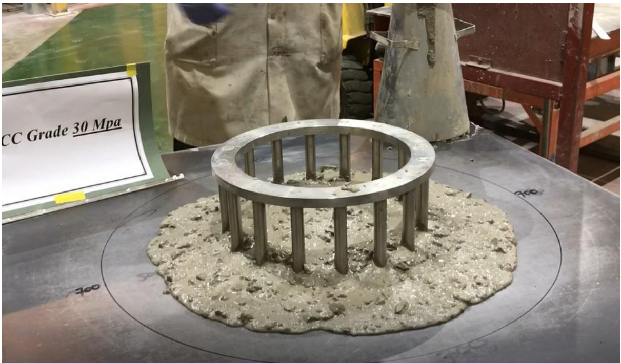
Figure C-1:Flowing and passing ability of SCC mix: C30
