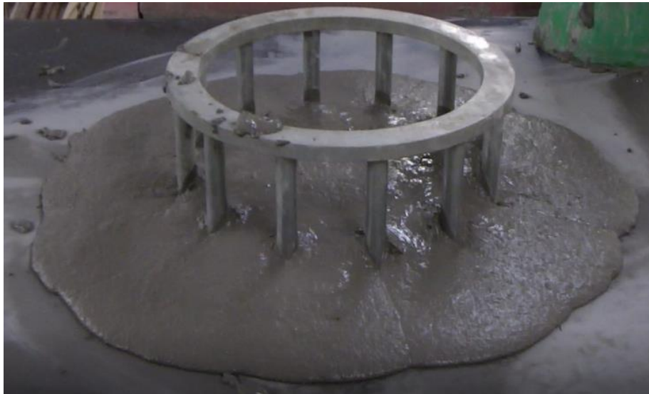
Figure 7.14: Flowing and Passing ability of SCSFRC mix (1%) volume (C30) Mix 3(4)
