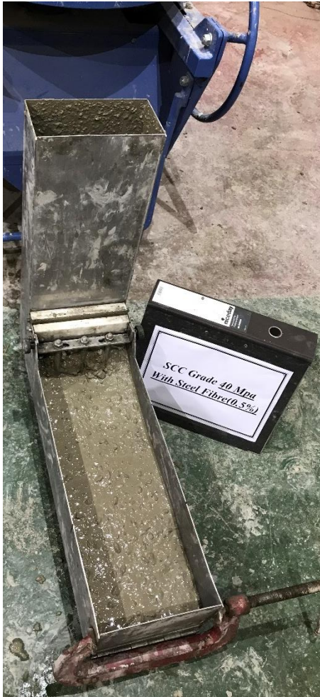
Figure C-8: Flowing , passing and filling ability of SCSFRC mix: C40
