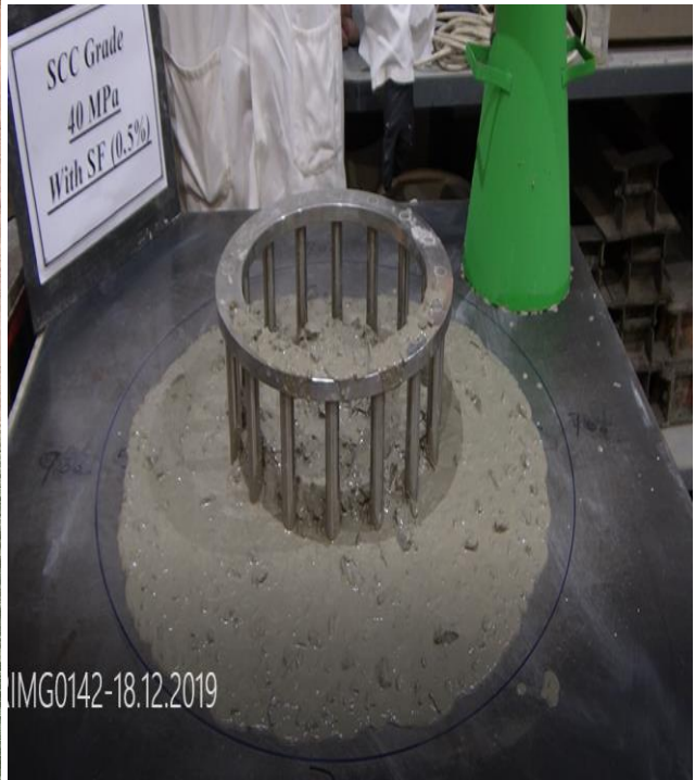
Figure C-8: Flowing , passing and filling ability of SCSFRC mix: C40
