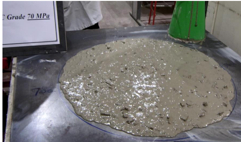
Figure 6.5: Horizontal spread of SCC mix C70
