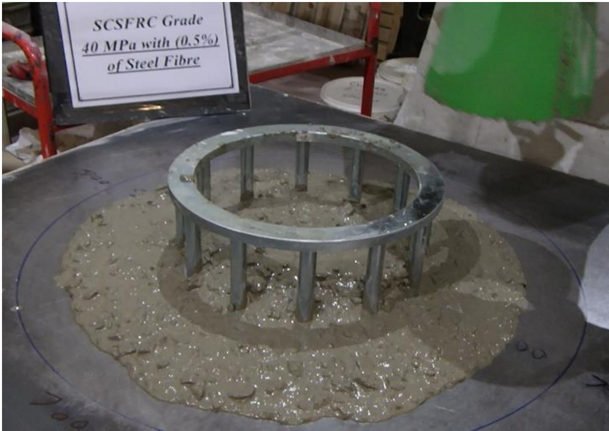
Figure C-9:Flowing and passing ability of SCSFRC mix: C40
