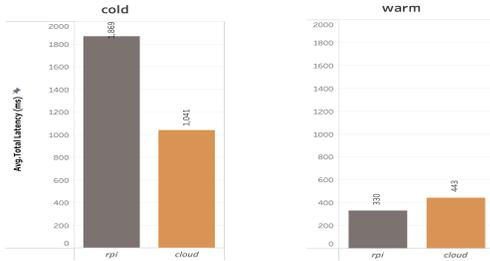
Fig. 10: Average latency: F3\_PRIME in cold/warm activation
