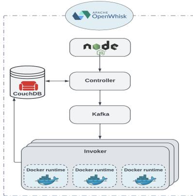
Fig. 1: Apache OpenWhisk architecture
