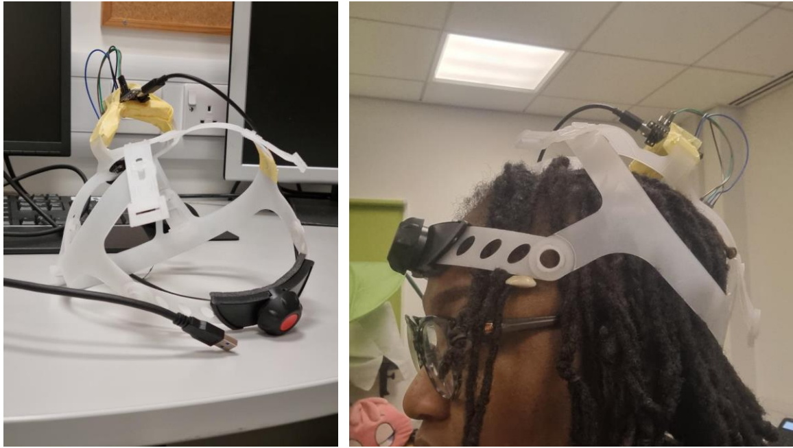
Figure 6-1: Device designed to measure head orientation
