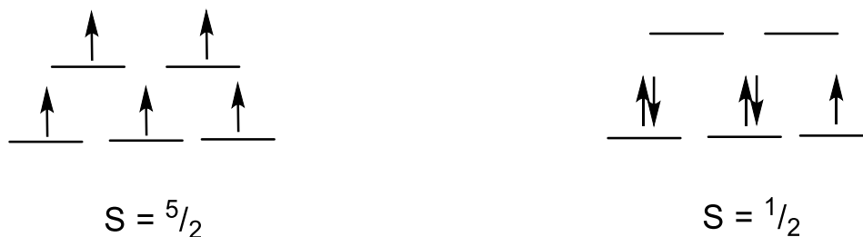
Figure 2.32 MO diagram of both spin states observed for octahedral Fe(III) complexes, namely S = 5/2 and S = 1/2 .
