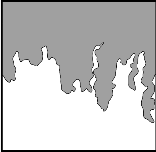
Figure 6.1: A slice obtained from MRI imaging of a 15 \times 15 \times 15 \text{ cm}^3 sand sample showing a fingered profile after having 600ml of water introduced over 3 minutes to the top surface (after Posadas Ay et al. (1996))
