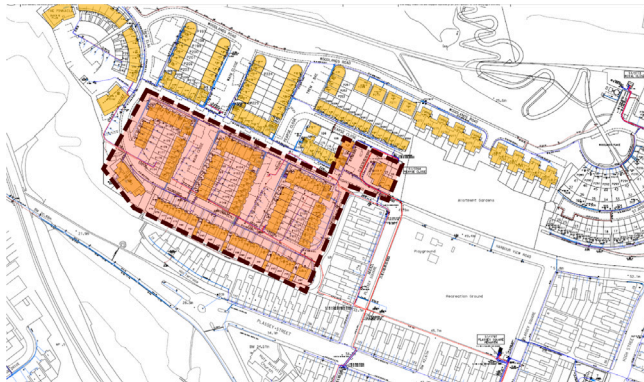
Fig. 13. The power network layout for the case study area in the Vale of Glamorgan, UK.
