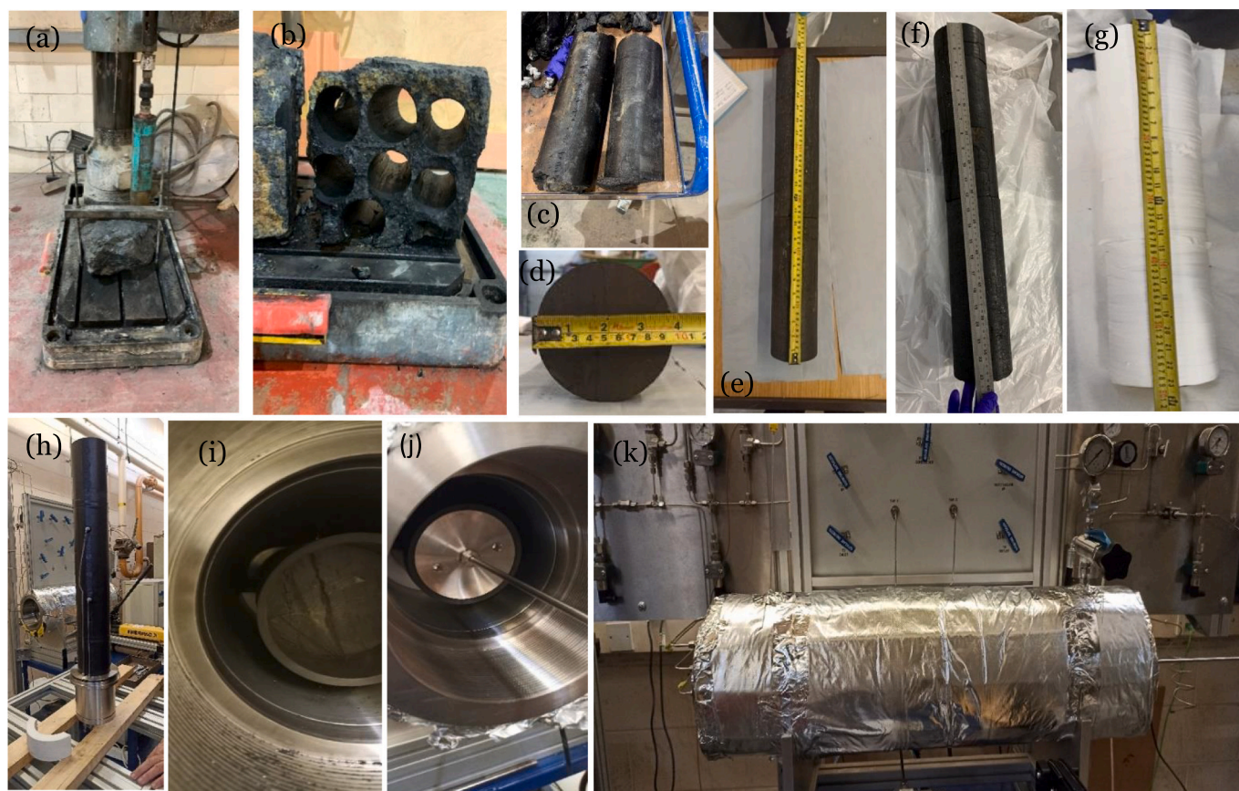
Fig. 2. (a) Core drilling equipment, (b), (c) and (d) 9.9 cm diameter cores drilled out of large blocks, (e) EMB coal cores, (f) ZM coal cores, (g) cores wrapped in PTFE tapes, (h) Viton tube with pressure taps, (i) Viton tube with cores inserted and placed inside the core holder, (j) the gas tight plunger with gas outlet tube inserted to the Viton tube, and (k) the experiment ready hydrostatic core holder set up.
