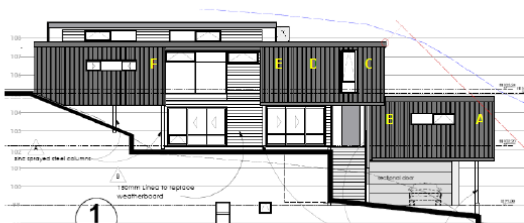
Figure 36. Elevation and location of TSC cladding (22).
