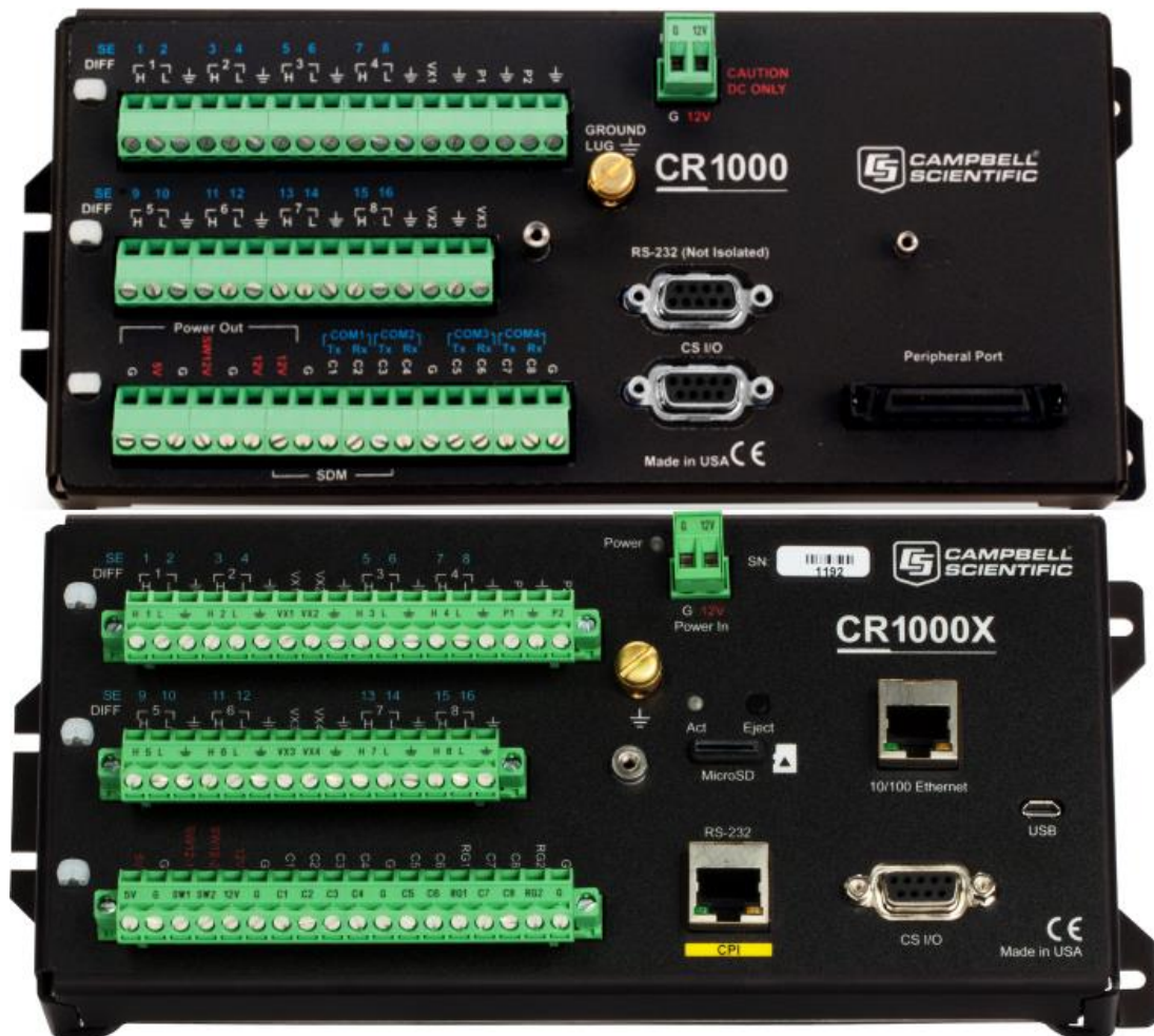
Figure 7-44 CR1000 (up) and CR1000X (bottom); the data logger from Campbell Scientific used in all the experimental case studies, author.
