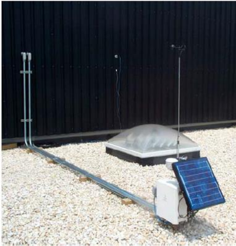
Figure 18. Data acquisition system with TSC in background (9).
