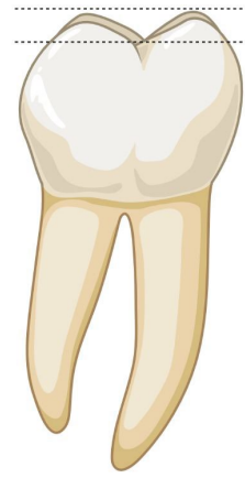
Fig. 5. Whole tooth with the top surface measurement region limitation of the optical (CFS) method, with dotted lines representing the sensor gauge range.
