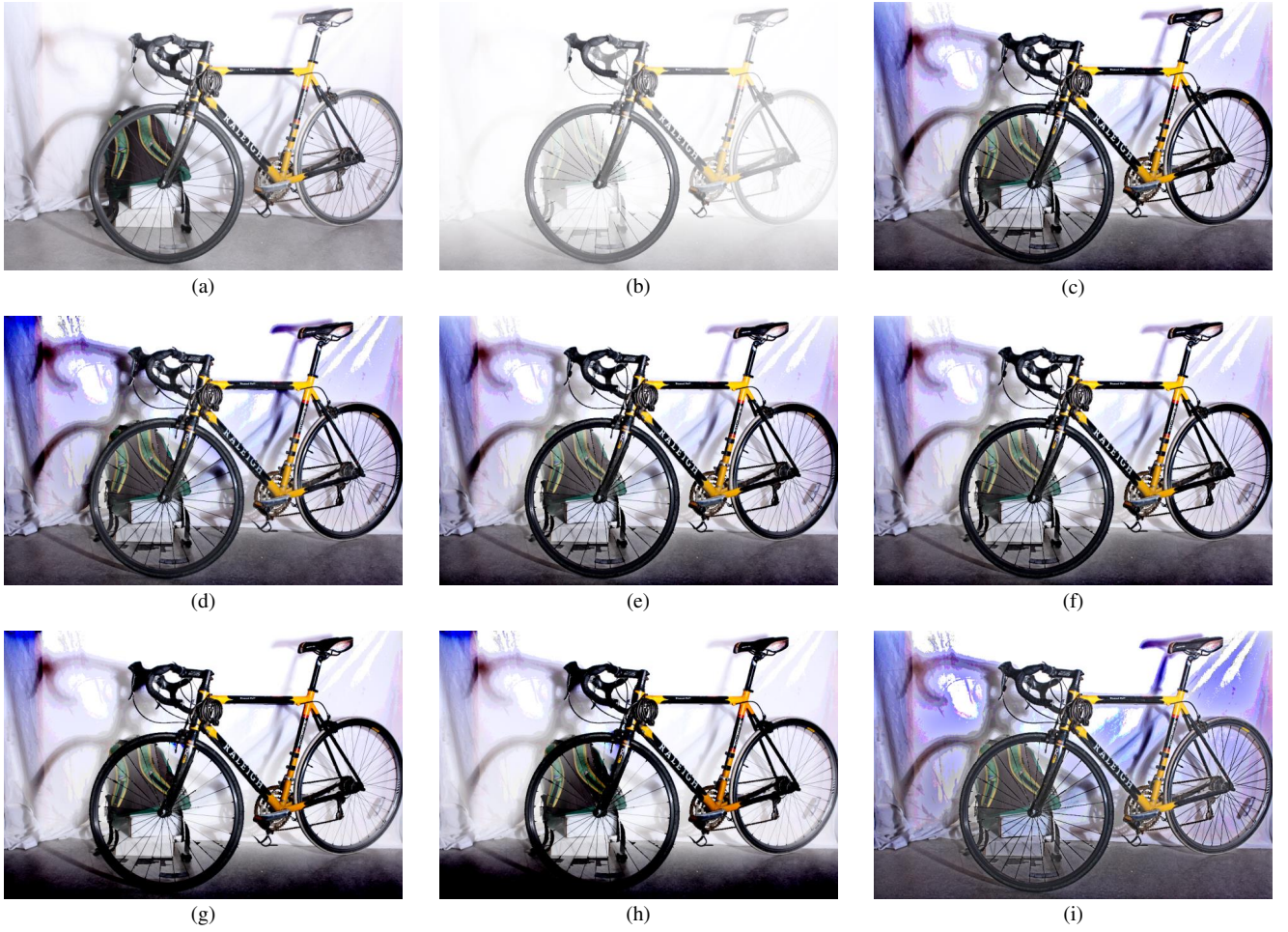
Fig. 11: Image dehazing by using different parameters. (a) A reference haze-free image; (b) The corresponding hazy image; (c) Dehazed image with default parameters, i.e., \alpha = 0.5 , \lambda = 1.0 and Q_{RRPD} = 38.8803 ; (d) Dehazed image with \alpha = 0.05 , \lambda = 1.0 and Q_{RRPD} = 54.1494 ; (e) Dehazed image with \alpha = 5 , \lambda = 1.0 and Q_{RRPD} = 34.8126 ; (f) Dehazed image with \alpha = 50 , \lambda = 1.0 and Q_{RRPD} = 34.1356 ; (g) Dehazed image with \alpha = 0.5 , \lambda = 0.1 and Q_{RRPD} = 26.9847 ; (h) Dehazed image with \alpha = 0.5 , \lambda = 0.01 and Q_{RRPD} = 32.0869 ; (i) Dehazed image with \alpha = 0.5 , \lambda = 10 and Q_{RRPD} = 81.1083 .
