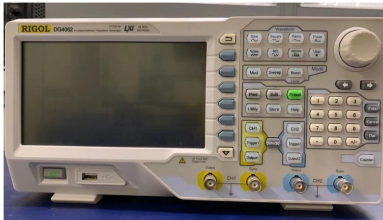
Fig. 5.18. RIGOL DG4062 series wave generator.
