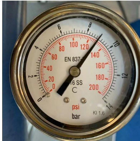
Fig. 5.4. Analog pressure gauge from 1-15bar(abs.).
