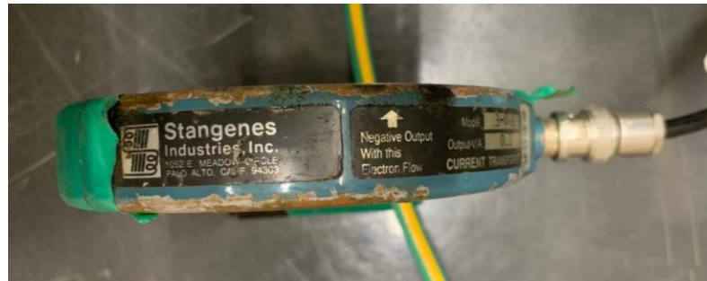
Fig. 5.14. Stangenes Industries inc. 3-0.1 series CT.
