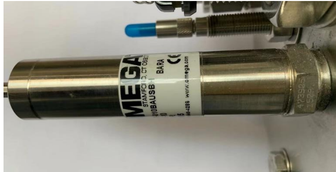
Fig. 5.6. OMEGA built-in pressure sensor.
