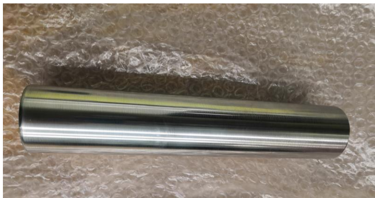
Fig. 5.3. Inner conductor (HV electrode tube) for GIL prototype.
