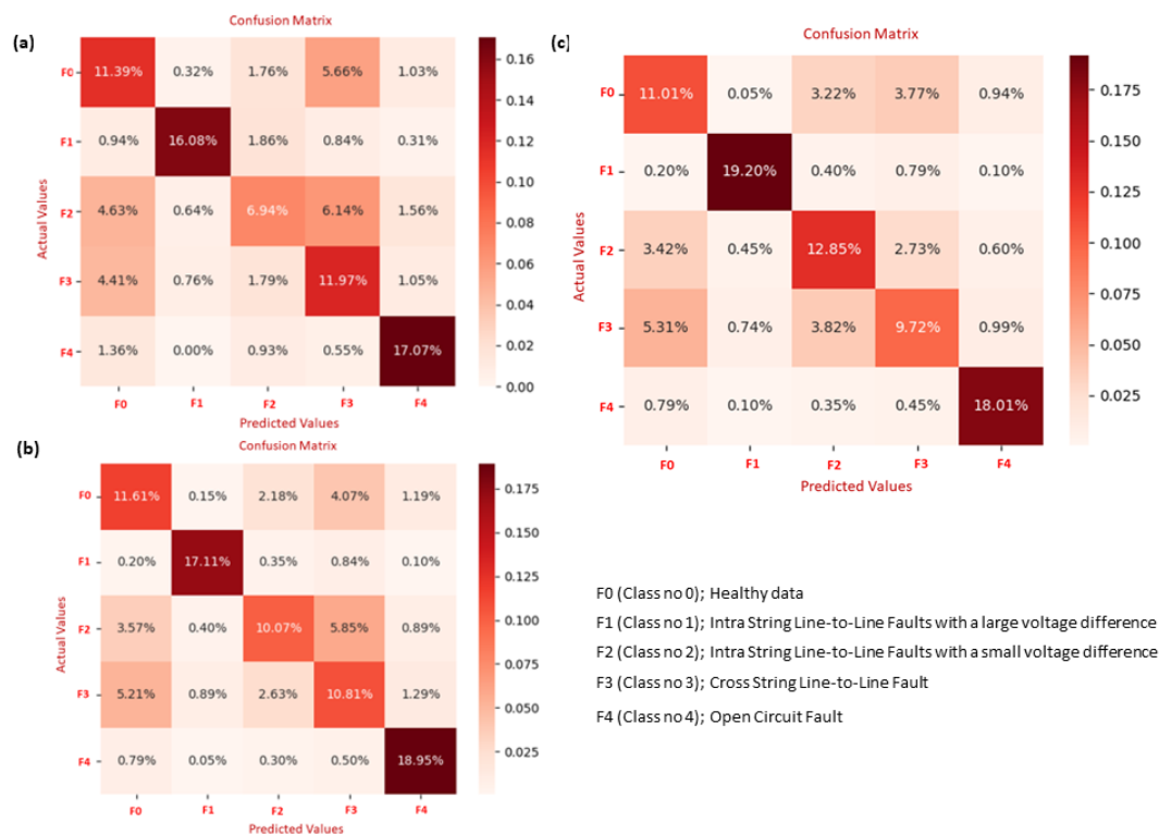
Figure 10. Confusion matrix illustrating fault identification based on classifiers: (a) SVM, (b) SVM-PSO, and (c) SVM-BA.
