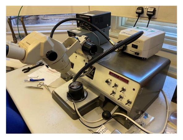
Figure 33:West Bond wire bonder used for gold-to-gold contacts.
