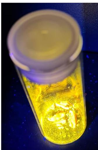
**Figure 5.5:** Photograph of poly(EDHP-CHO-PA) after its complexation to in  $[\{\text{Ir}(\text{PhPy})_2\mu\text{-Cl}\}_2]$ , taken during its exposure to UV light. The orange/yellow glow is indicative of iridium, and contrasts strongly to the off-white polymer seen pre-complexation and the pale yellow colour of the iridium precursor.
