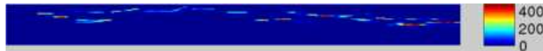
(c) Grid with each cell containing the number of 3D points projected on it
