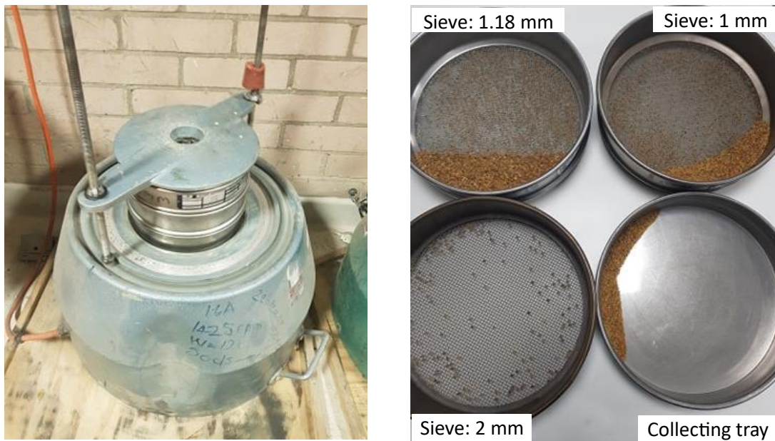
Figure 3.6: Electro-mechanical sieve shaker. Sediment was put through the sieve process for 10 minutes, with progressively smaller graded sieve mesh to obtain the average particle size and range. When the sediment distribution was obtained this was checked against the particle standards to ascertain the correct grade of sediment. Sediment range displayed in Table 3.1.
