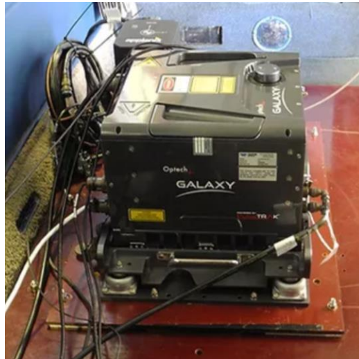
Figure 6.2: Photograph displaying an Optech Galaxy with integrated Optech LW640 Thermal Camera mounted to a surveying aircraft (BlueSky, 2021).
