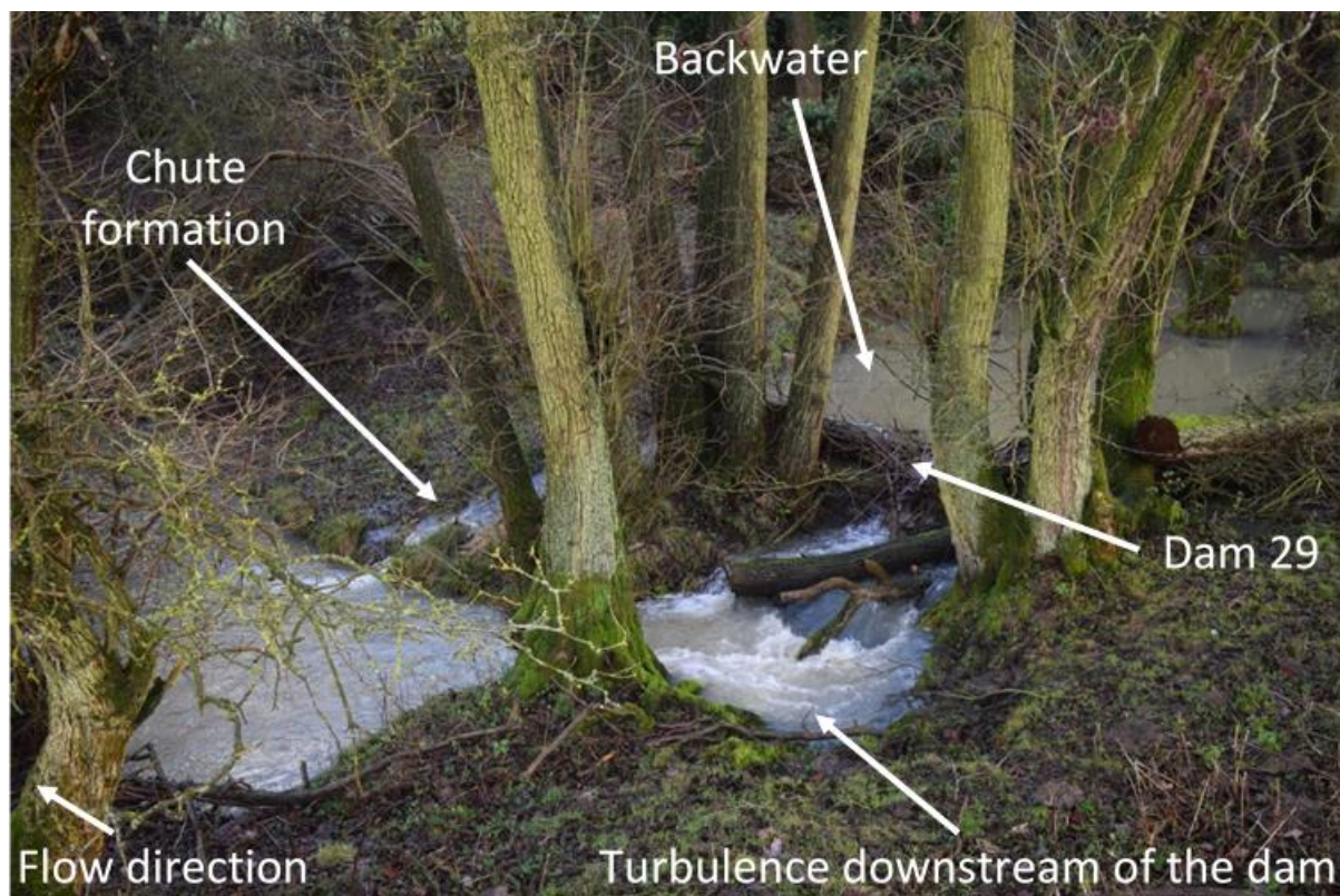
Figure 5.20: Shows a chute and meander remaining simultaneously active. During high discharge, dam 29 has caused the flow to overtop the channel bank and form a chute across the meander neck. This process of channel blockage caused by a WDD is corroborated by Keller and Swanson (1979). The chute diversion can reduce the main channel capacity with enhanced shoaling until eventually the chute becomes the sole flow route (Pinter et al., 2004). However, Grenfell et al. (2012) report partitioned meanders and chutes can continue to co-exist for decades. Photograph by Neden (21 December 2018).
