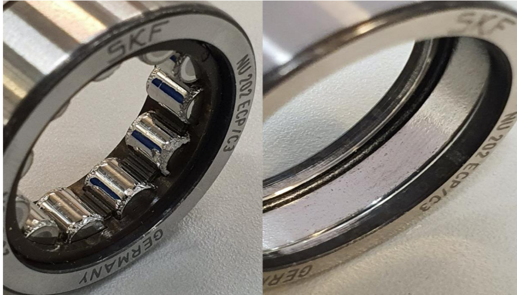
Figure 6-35: First SKF NU202ECP/C3, damage sustained on rollers and outer raceway.
