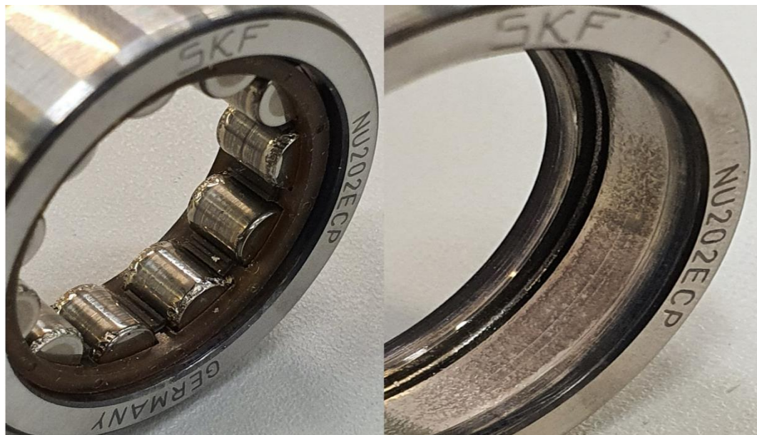
Figure 6-33: Second SKF NU202ECP, damage sustained on rollers and outer raceway.
