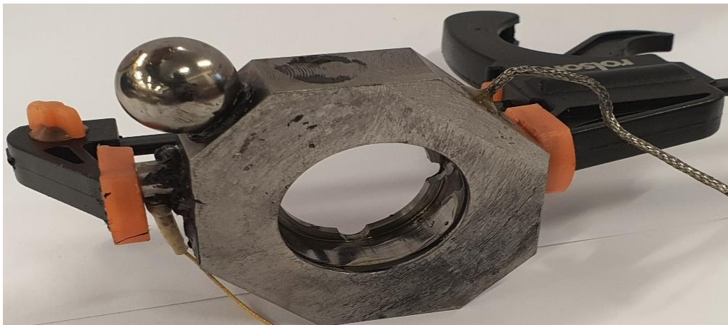
Figure 4-7: AE Sensor mounted on the test bearing housing and held with a clamp for 24 hours.
