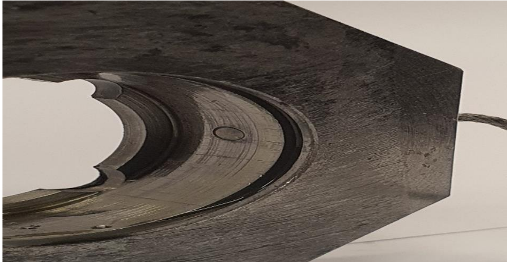
Figure 4-10: Thermocouple location on the outer raceway of the test bearing housing.
