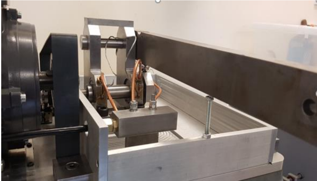
Figure 4-5: Two support Bearings on the left hand side of the modified High-Speed Test Rig.
