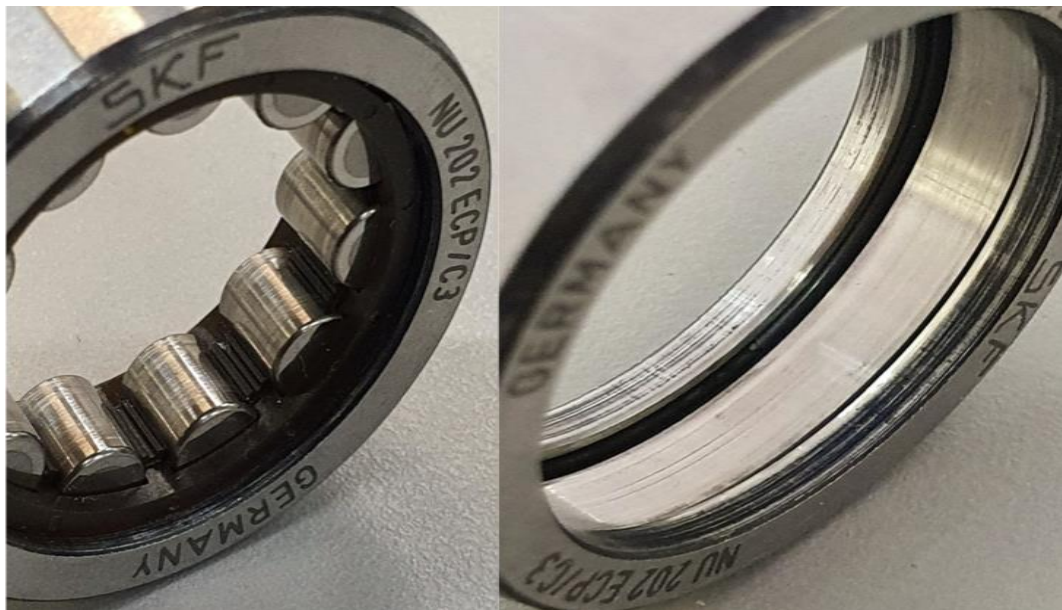
Figure 6-37: Second SKF NU202ECP/C3, damage sustained on rollers and outer raceway.
