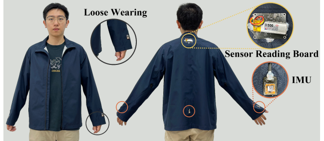
Figure 2. Prototype demonstration of the loose-wear jacket embedded with IMU sensors and the circuit board for data collection.
