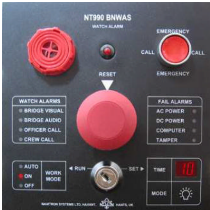
Figure 3: Example of a BNWAS bridge panel
