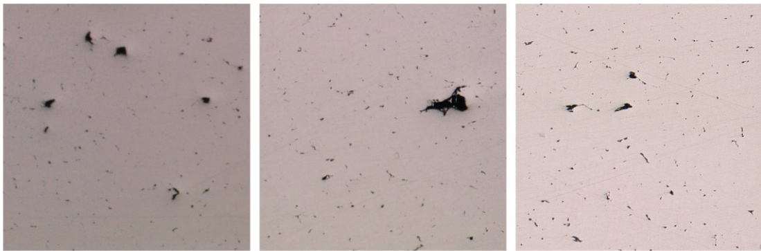
Figure 6.7 Examples of LOM images for porosity detection in the dataset
