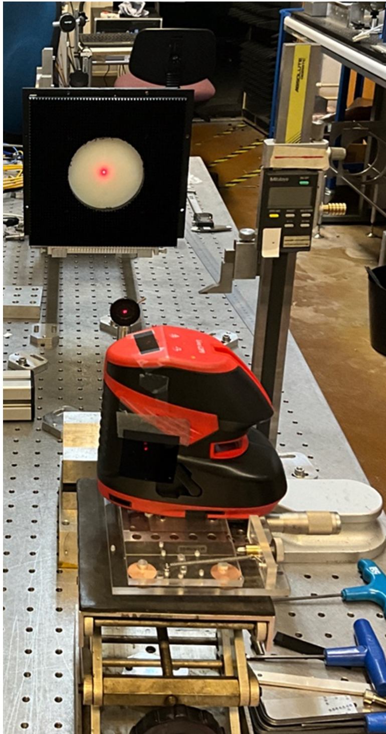
Figure 4.20 – Laser aligned to aperture and target with lens inserted to measure position of laser dot with respect to the centre of the lens. On the lens the centre is marked by a black dot. The lens is at the front of the lens mounting structure here.
