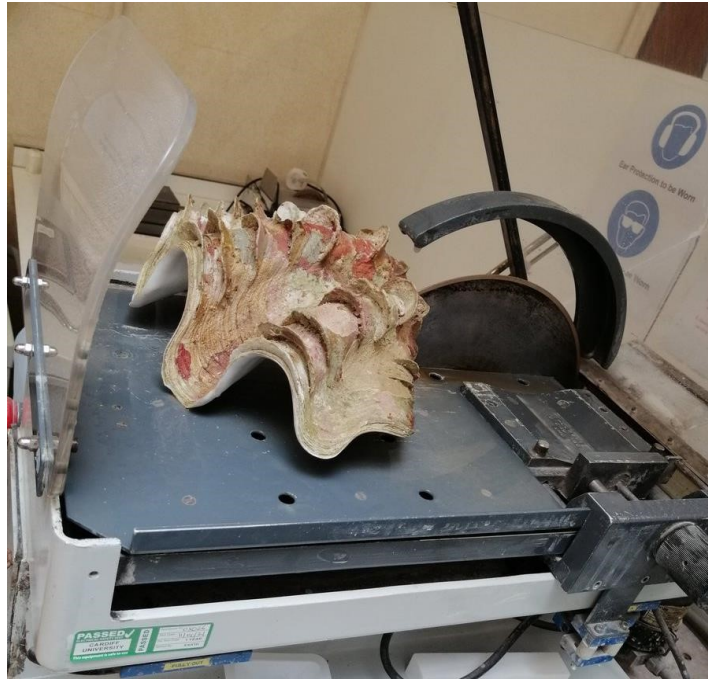
Figure 2.24. Tridacna squamosa shell valve on platform of diamond saw apparatus, in preparation for cutting longitudinally along the axis of maximum growth.
