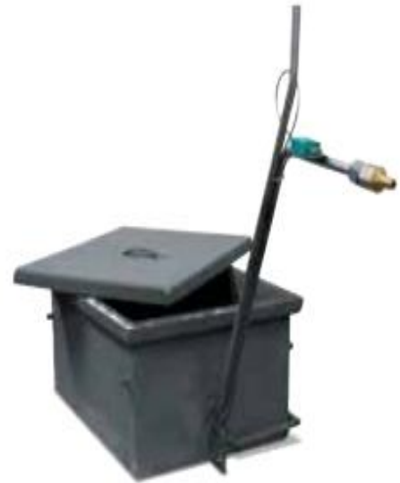
Figure 3-6 Box for a protective gas atmosphere using a charging cart.
