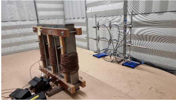
Fig. 3. Conventional nine microphone array test arrangement placed 70cm from the transformer.
