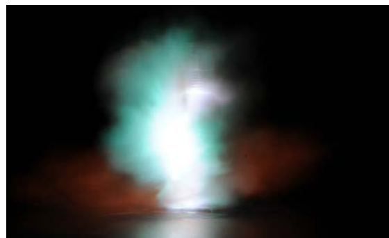
Fig 4. An image of a 55.5 kA lightning arc taken with a shutter opening time of 6 s.
