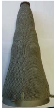
Figure 2.8: AM manufactured Ku-band spline horn antenna. Reprinted from[48].
