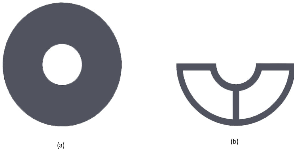
Figure 3.16: PTFE spacer design a) is a solid design, and b) is a half spacer with voids in the structure, reducing dielectric loss.
