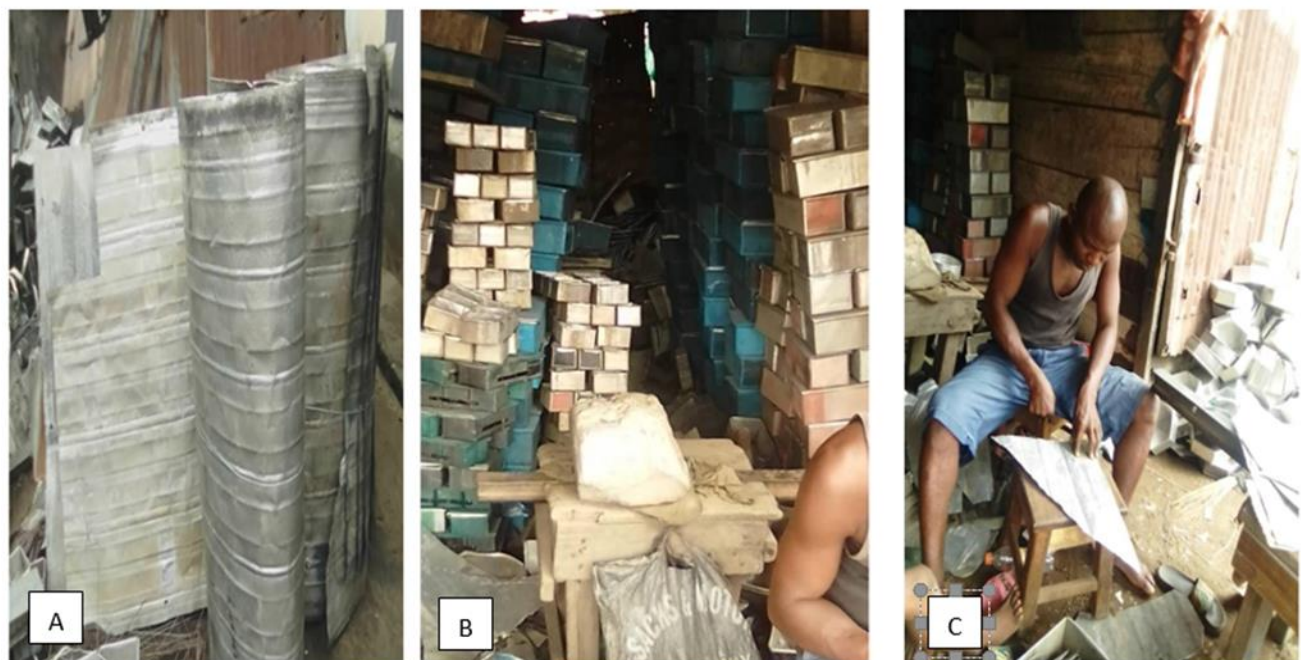
Figure.6.5 Aluminum waste being worked on to create baking pans (© Researcher's proxy field work, 2021).
