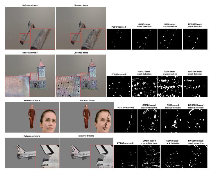
Fig. 3. Crack maps of local windows of four different input pairs of reference and distorted frames obtained from the Nehmé *et al.* [13] (first two rows) and TSMD [17] (last two rows) datasets. GMSD [18], SSIM [19], and IW-SSIM [20] quality maps are also generated and binarized with optimized thresholds and added as baselines for comparison with the proposed PCD method.
