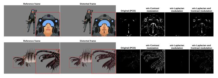
Fig. 4. Ablation study for contrast and Laplacian modulation components of the proposed PCD method for two sets of input pairs of reference and distorted frames obtained from the TSMD dataset [17].
