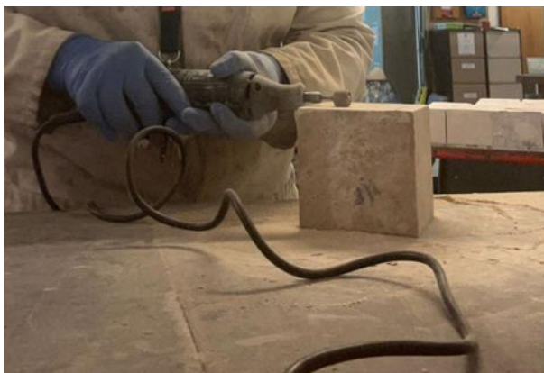
b) Hand grinding was used to achieve the SP2 grade
