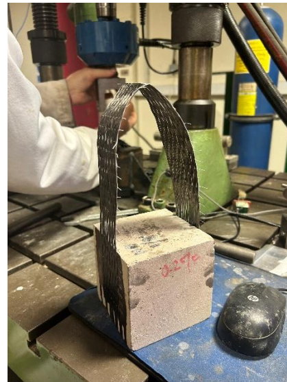
b) CFRP installed sample
