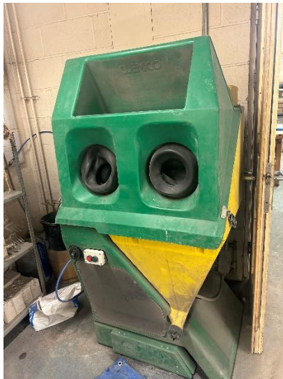
b) Sand blasting machine in the concrete lab
