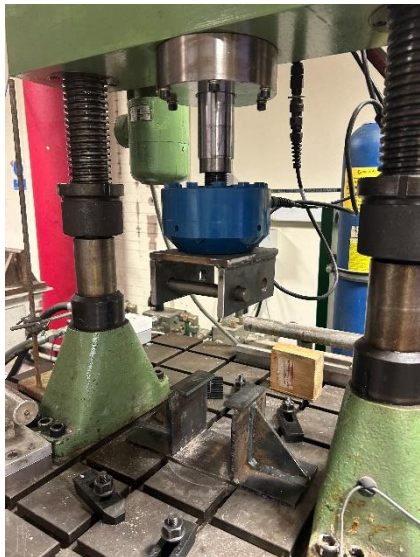
a) steel cage used to place sample and the universal hydraulic test machine
