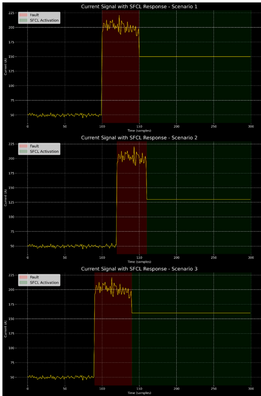
Fig. 23. Current Signal with SFCL responses in different scenarios.
