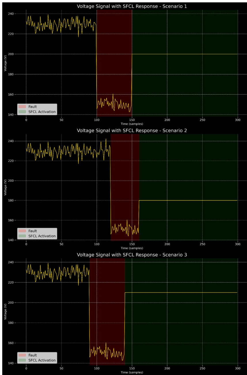
Fig. 24. Voltage Signal with SFCL responses in different scenarios.
