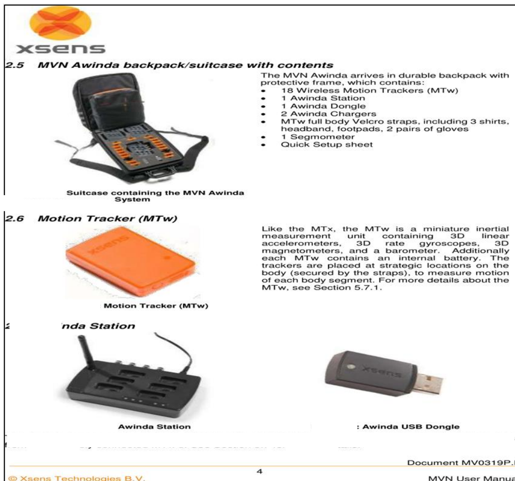
Figure 4: MVN Awinda suitcase and contents (MTw, Awinda station, USB dongle) adapted from Xsens Technologies B.V. (2021).
