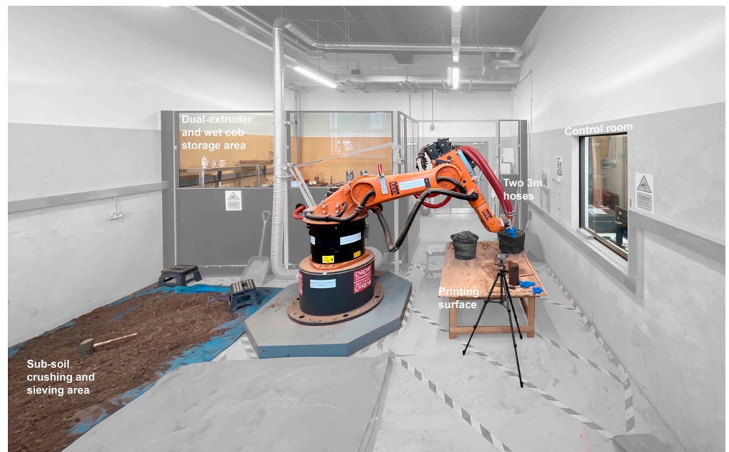
Figure 1. Robotic lab working areas. The length of the two hoses connected to the two-way aluminium channel held by the robot influences the distance the wet cob travels and, consequently, the required extruding force.
