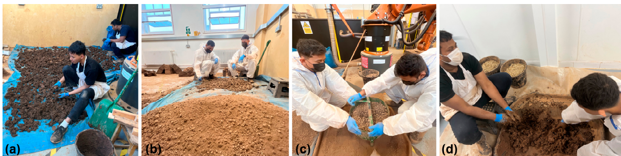
Figure 6. The dry cob-like mixture preparation process involves a series of steps depicted from left to right: (a) Spreading the wet subsoil for drying. (b) Sorting and pulverising the dried subsoil using rubber mallets. (c) Sieving the crushed subsoil through a 10 mm sieve. (d) Combining the sieved subsoil with cut straw to produce the cob-like dry mixture. Water is subsequently introduced to yield the cob-like wet mixture.
