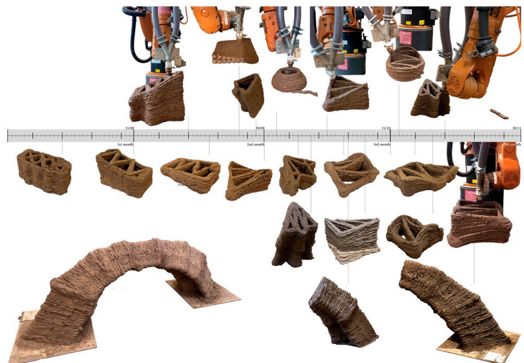
Figure 11. Nonplanar spatial prototypes are presented in the chronological order of printing over a four-month period. Selected parts were assembled into an arch.
