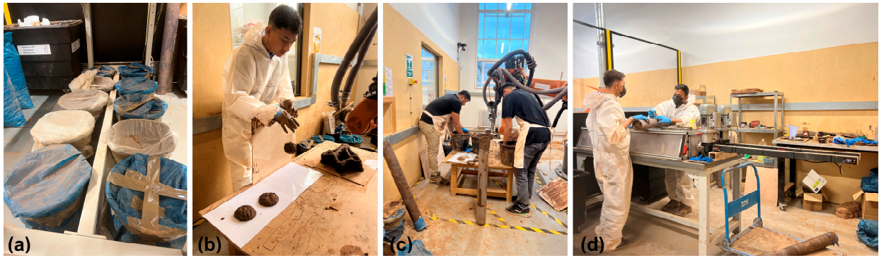
Figure 7. The wet cob-like preparation process encompasses four sequential steps: (a) Once water is added, the wet cob-like mixture is stored in sealed buckets. (b) The water quantity is readjusted using a controlled grid-measured drop ball test. (c) The wet cob-like mixture is loaded into the tubes and manually compressed and compacted. (d) The tubes are then loaded into the bespoke extruder, which is part of the continuous cob robotic printing process.
