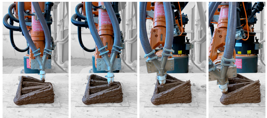
Figure 10. Extruded material is deposited perpendicularly to the toolpath of the printed geometry.
