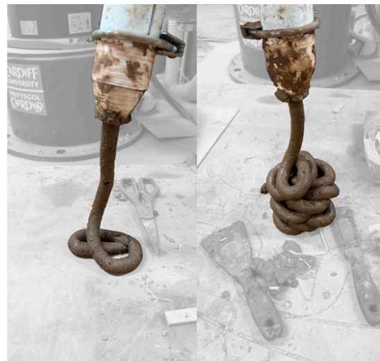
Figure 9. The substitution of a traditional sausage soil test with a robotic sausage-like extrusion to check wet-cob material consistency and buildability.
