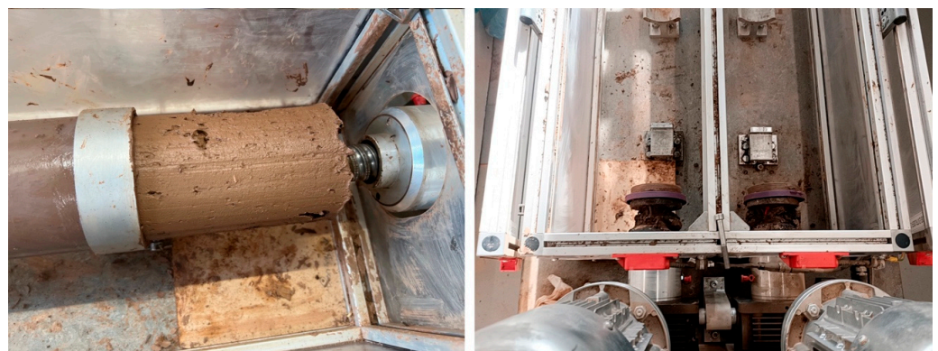
Figure 2. The rubber seal was added to the extruder's push plate to force the material forward movement.
