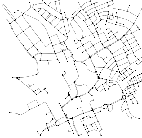
Figure 1: The street network of central Cardiff, Wales. Vertices and arcs are represented by black dots and grey lines respectively.
