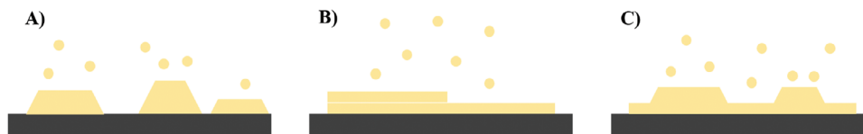
Figure 13. Different types of thin film growth, A) Volmer-Weber, B) Stranski-Krastanov, and C) Frank-van der Merwe. It can be seen that the incoming particles (yellow) interact with the substrate (grey) and form either films or islands depending on each growth method.
