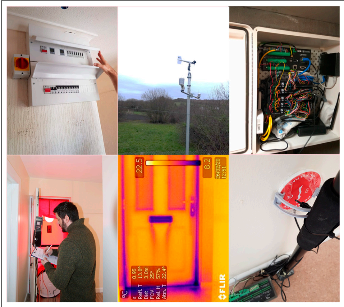
Figure 4. Top left - consumer unit with DIN rail meters, top centre – weather station, top right – logger and peripherals, bottom right – airtightness test, bottom centre – thermography during depressurisation, bottom right – U value measurements (credit: CLCBE team).
