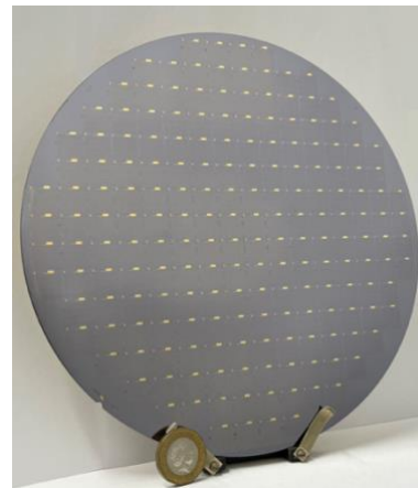
Fig. 1: A completed 200-mm VCSEL wafer. Each wafer contains 250,000 VCSEL devices.
