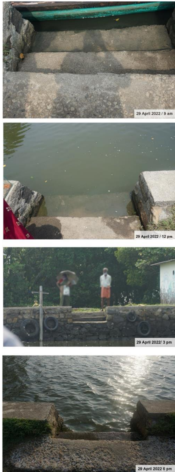
Figure 8.6: Change in water level due to tide in EMI based on the observation made on the islands in April, a difference of approximately 70-80 cm in water level due to tide was noticed.
