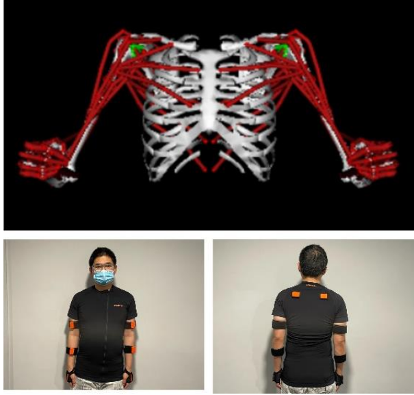
Figure 3. The upper limb musculoskeletal model and a participant are equipped with Xsens IMU sensors for demonstration.
