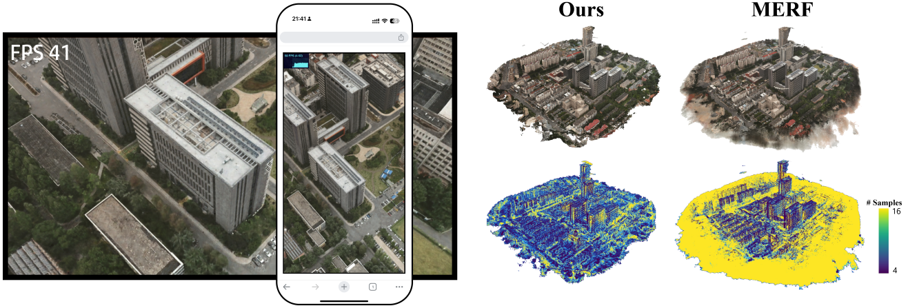
Figure 1. Oblique-MERF enables real-time synthesis of novel views for oblique photography on diverse commodity devices, including tests on an NVIDIA GTX 1650 ( \sim 41 FPS) and an iPhone 14 Pro Max ( \sim 45 FPS) (left). We introduce a novel compact sampling representation that markedly reduces sampling points and emphasizes significant regions, enhancing rendering quality and increasing frame rates. We present the rendering output and the visualization of the number of samples (right).
