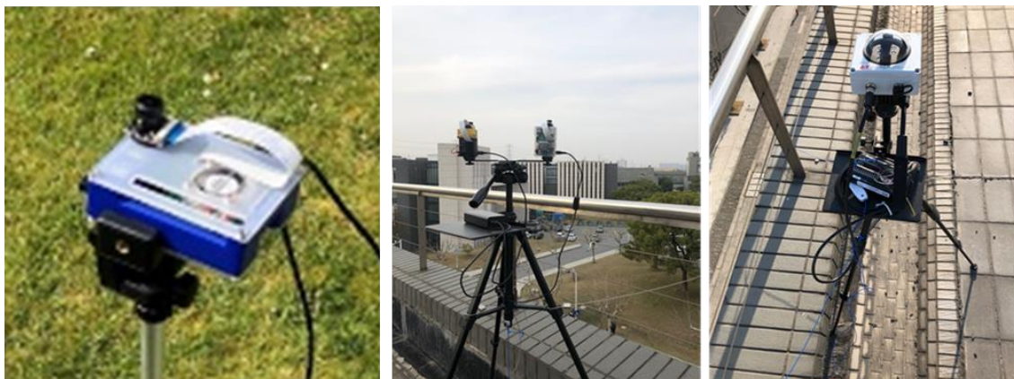
Figure 3.2 Raspberry Pi total sky imager (Left 1 and 2), BF5 sunshine sensor (Right).
