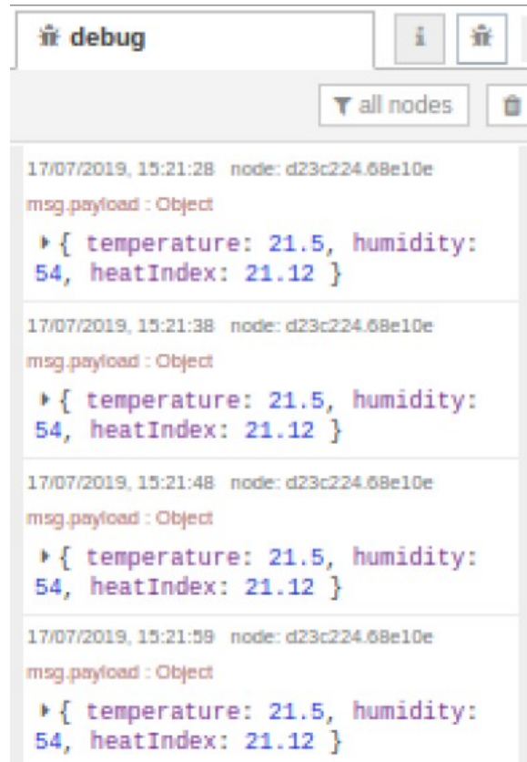
Figure 2.7: Debug Window Showing Temperature/Humidity Values
