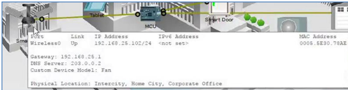
Figure 7.4: Viewing Device Information in a Smart Home Network
