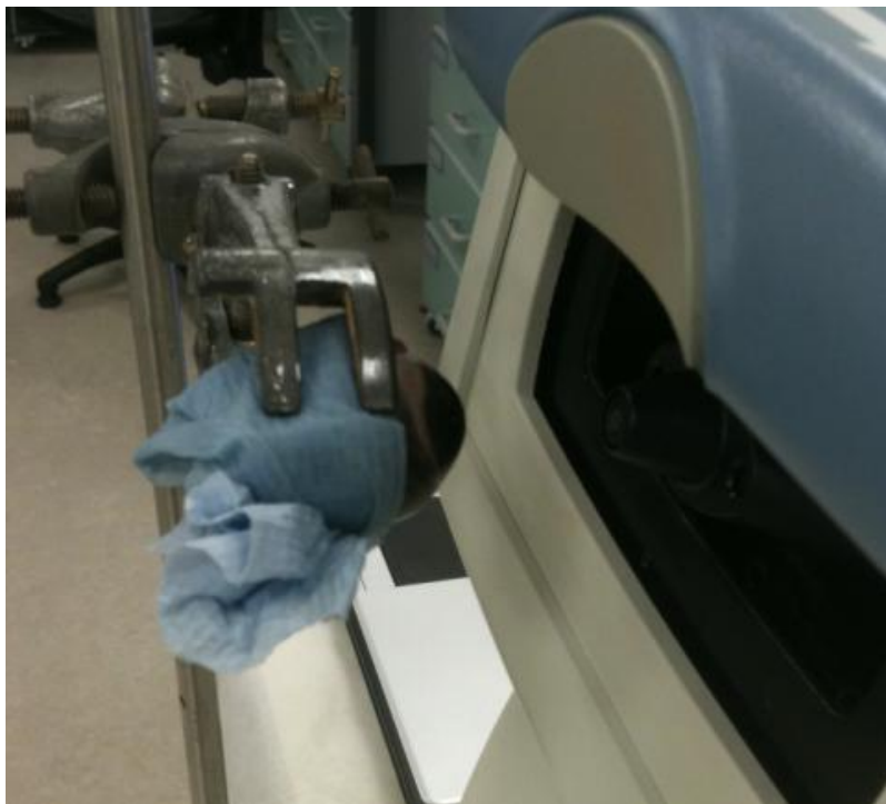
Figure 2.3: A fresh eye during the measurement in front of the ORA
