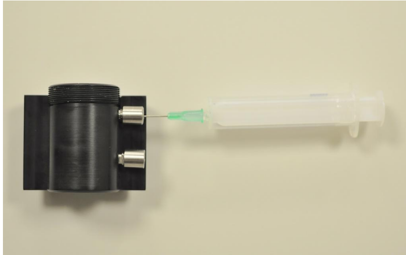
Figure 2.12: T syringe inserted through the valve in the chamber
