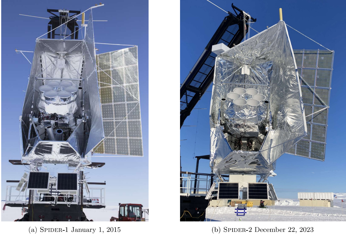
Figure 2: Photos of the fully integrated SPIDER-1 and SPIDER-2 payloads before their respective launches. Some key components visible in the photographs are the solar panels, star cameras, electronics, telescope forebaffles, and the sunshield. SPIDER-1 photo from Jon Gudmundsson.
