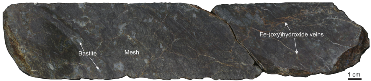
Fig. S14: Highly weathered and serpentized peridotite. Fe-(oxy)hydroxide veins locally reuse former serpentine veins and cut through the serpentine-magnetite veins (mesh network) and bastite suggesting weathering postdates serpentinization (Interval 399-U1601C-27R-1, 28-55 cm).
