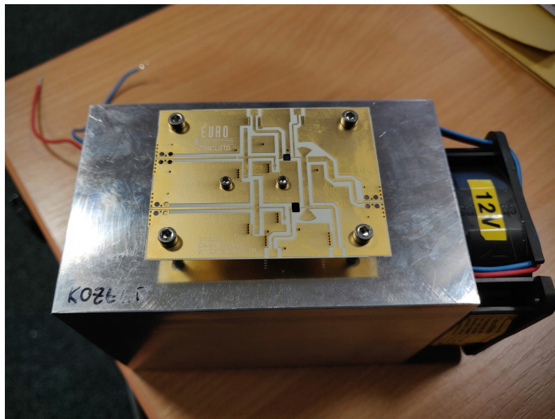
Figure 5.2: Dual Input Doherty test fit on heatsink
